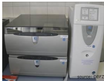
Figure 9: Analyzer for S & Cl according to EN o 15289 (source: DBFZ)
