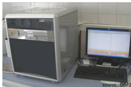
Figure 10: CHN-analyzer according to EN o 15104 (source: DBFZ)
