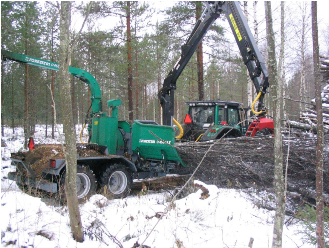
Figure 4. Chipping of delimited trees or whole trees by Kesla drum chipper.
