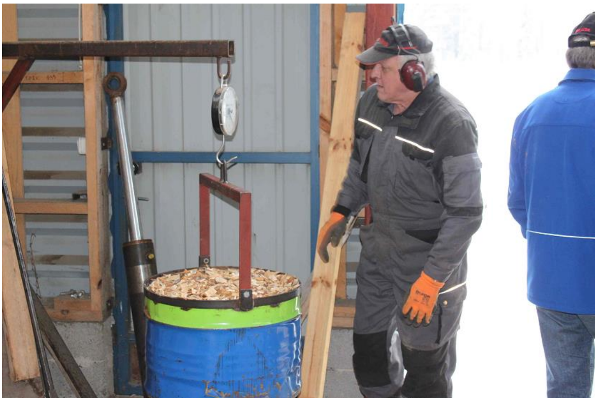
Figure 6. Truck driver Mauno Uusimäki is measuring the bulk density of the wood chips.
