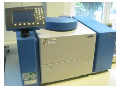
Figure 8: Bomb calorimeter according to method EN 14918 (Source: HFA)
