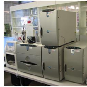
Figure 7: Analyzer for Cl according to method EN 15289 (Source: ENAS Oy)
