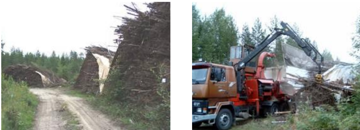
Figure 3: Whole tree piles covered by Kraft paper to protect them from rain and snow during storage; wood chipper (Source: VTT)
