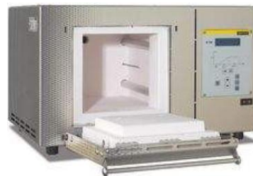
Figure 13: High temperature laboratory furnace according to method EN 14775 (Source: VTT)
