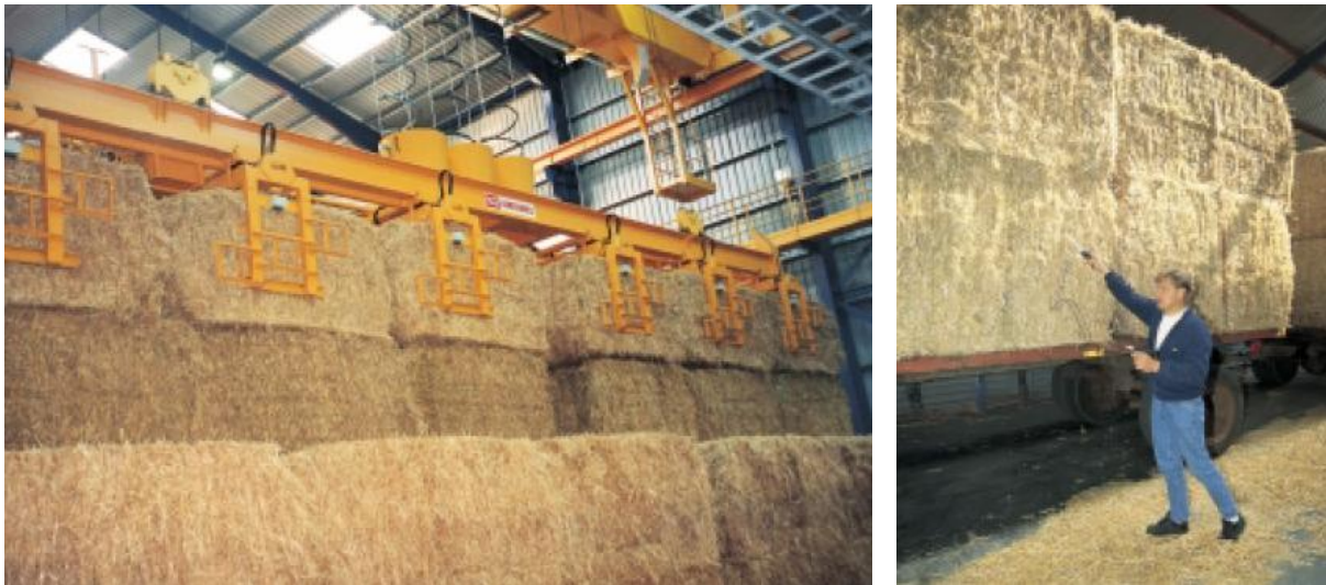
Figure 7: From the intermediate storage the bales are transported to an energy plant - the end user and unloaded in the storage. Usually, the bales are weighed and the moisture content is measured at this stage - either automatically (at large plants) or manually (Source: Sønderjyllands Højspændingsværk and BioPress/Torben Skøtt).
