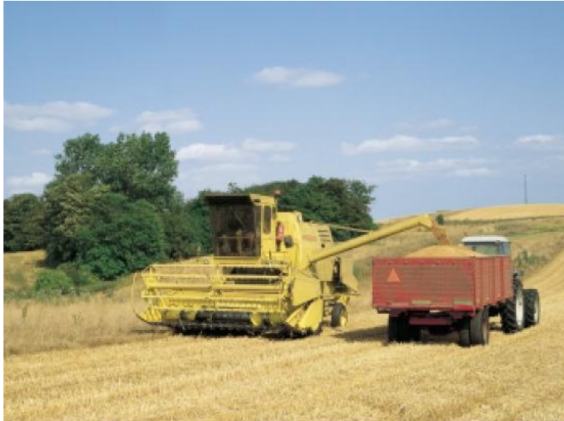
Figure 2: Cereal grain harvest - this harvester is equipped with a chaff cutter that has cut the straw to be ploughed back. The straw is normally left in the field behind the harvester (Source: BioPress/Torben Skøtt).
