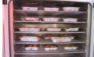
Figure 11: Drying oven according to method EN 14774-2 (Source: VTT)
