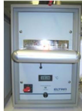
Figure 4: Analyzer for Cl according to method EN 15289 (Source:VTT)
