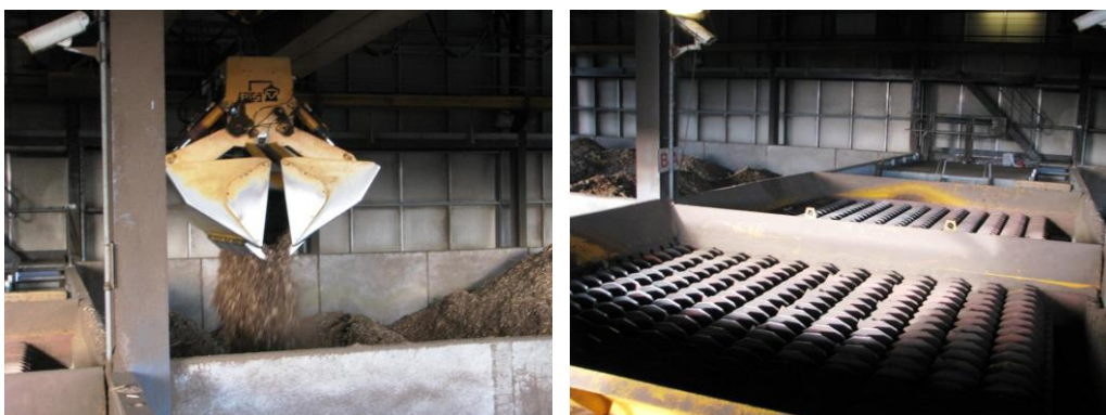
Automatic grab crane and rotating screens. (Photos: Morten Tony Hansen)
